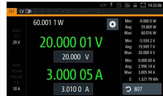
The large capacitive touchscreen is the central operating element on the R&S®NGM200. The very high resolution of 800 x 480 pixel makes it easy to read voltage and current values even from a distance. Information such as power values and statistics can be displayed in addition. Icons indicate the status of selected protection and special functions.
